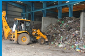
Waste picked up by front loaders/overhead grab cranes
